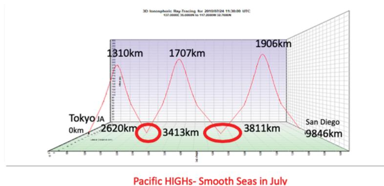
Figure 1 — PROPLAB 3-hop Tokyo – San Diego model for July 24, 2010, with superimposed data.
