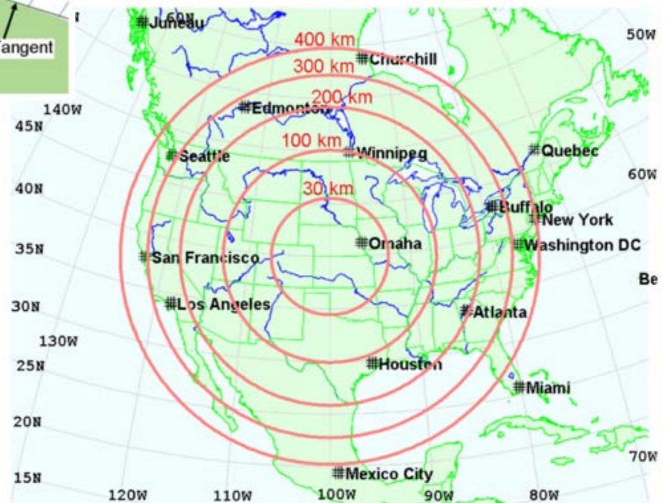
**Fig. 7** Samples of E1 HEMP exposed regions for several burst heights. The *red circles* show the exposed regions for the given burst heights, for a nuclear burst over the central US (from Savage et al. 2010)
