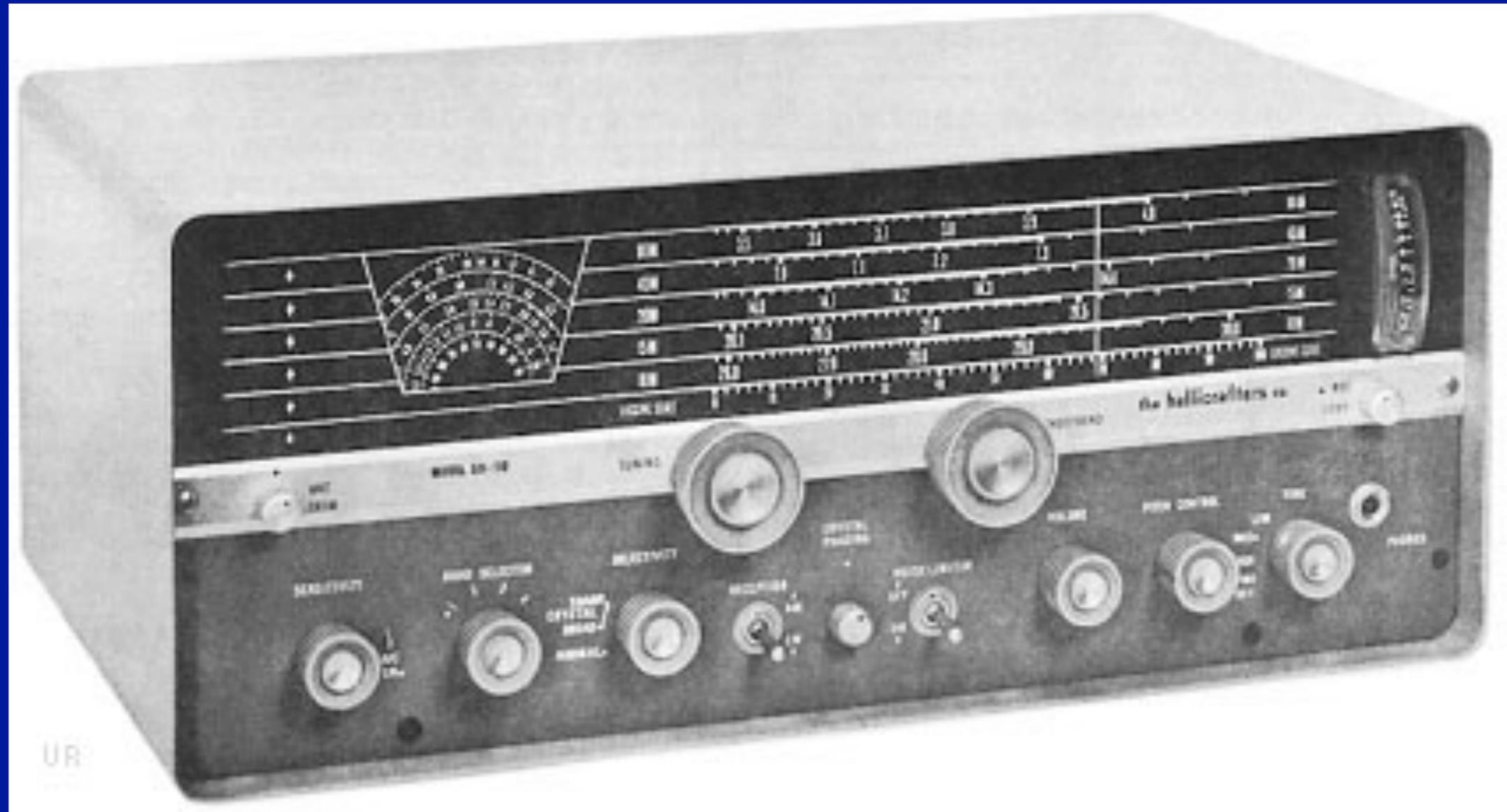
6SG7 RF Amp, 6SA7 Converter, 6SG7 1st IF Amp, 6SK7 2nd IF Amp, 6SC7 Audio Amp/BFO, 6K6GT Audio Output, 6H6 Detector/ANL/AVC and 5Y3GT Rectifier.
