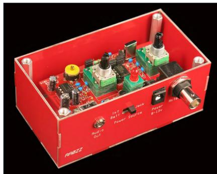
With many modifications, this evolved into the Grape I receiver. Note inputs for the GPS local oscillator and antenna, and output for the carrier mixed down to 1 kHz nominal.
