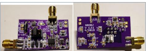
Grape II is also an NE612 low-IF receiver, but adds 3-frequency simultaneous reception, onboard frequency standards and A/D converters, improved filtering, microcontroller switching, and the most subtly toned LEDs N8OBJ could find.
