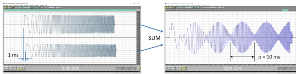
Fig 2a. Two 100 Hz/ms Chirps with 1 ms Time Delay. Delayed Chirp is 3 dB lower in Amplitude to Simulate Multipath.
