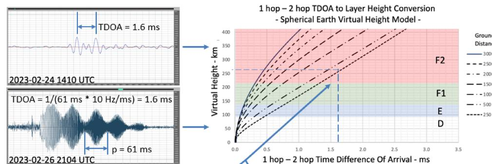
Fig. 3a Short Pulse and Chirp TDOA Measurements
