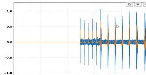
Fig. 2 The correlated result from the given tx3.wav file that enables us to find the starting point of each chirp
