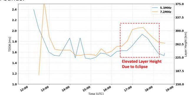
Fig 4. 5.3 and 7.3 MHz bands with their equivalent Layer Height. At 17:45 UTC the eclipse was at maximum annularity in Texas and the bumps correlate perfectly with the known times for the Austin ionosonde
