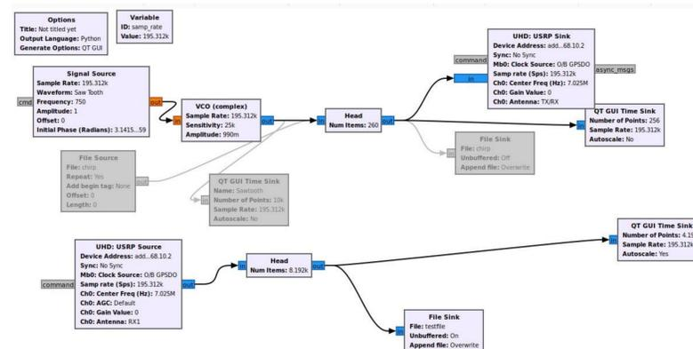
Figure 2. GNU radio flowgraph outputting a chirp and recording the return.
