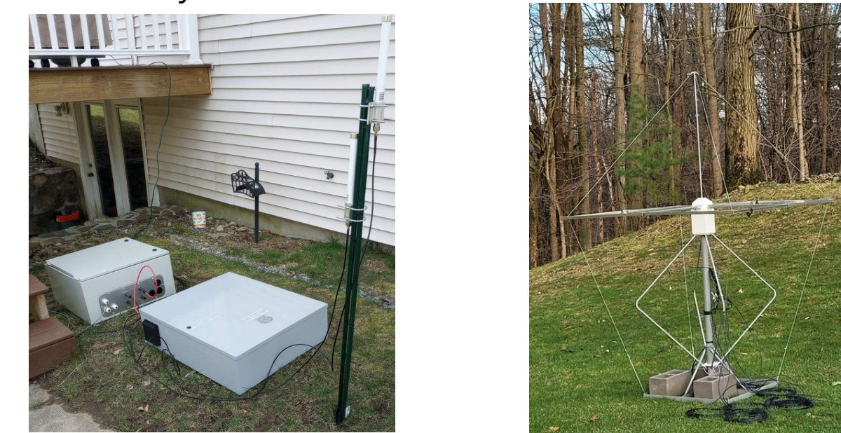
Below on the left, the radio and power system enclosures for the receiver. The right-hand side shows the EMVS antenna for this system.
